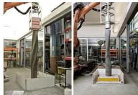
b) Smart Dynamic Casting process of slipforming, extruding concrete into a delimited formwork, controlled by a 6-axis robotic arm. Image: courtesy of Gramazio Kohler Research, ETH Zürich.
