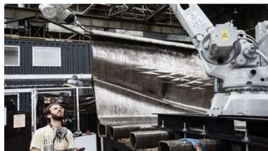
c) The MX3D's metal printer equipped with an industrial robot with an advanced welding machine, printing self-supporting steel bridge. Image: courtesy of MX3D.
