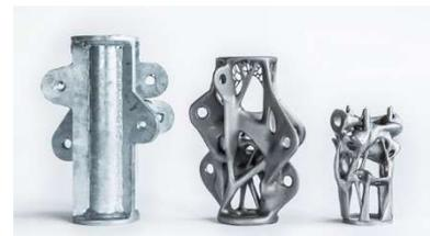
e) stainless steel nodes, topologically optimized and 3D printed in metal by Arup. Image: courtesy of Arup.
